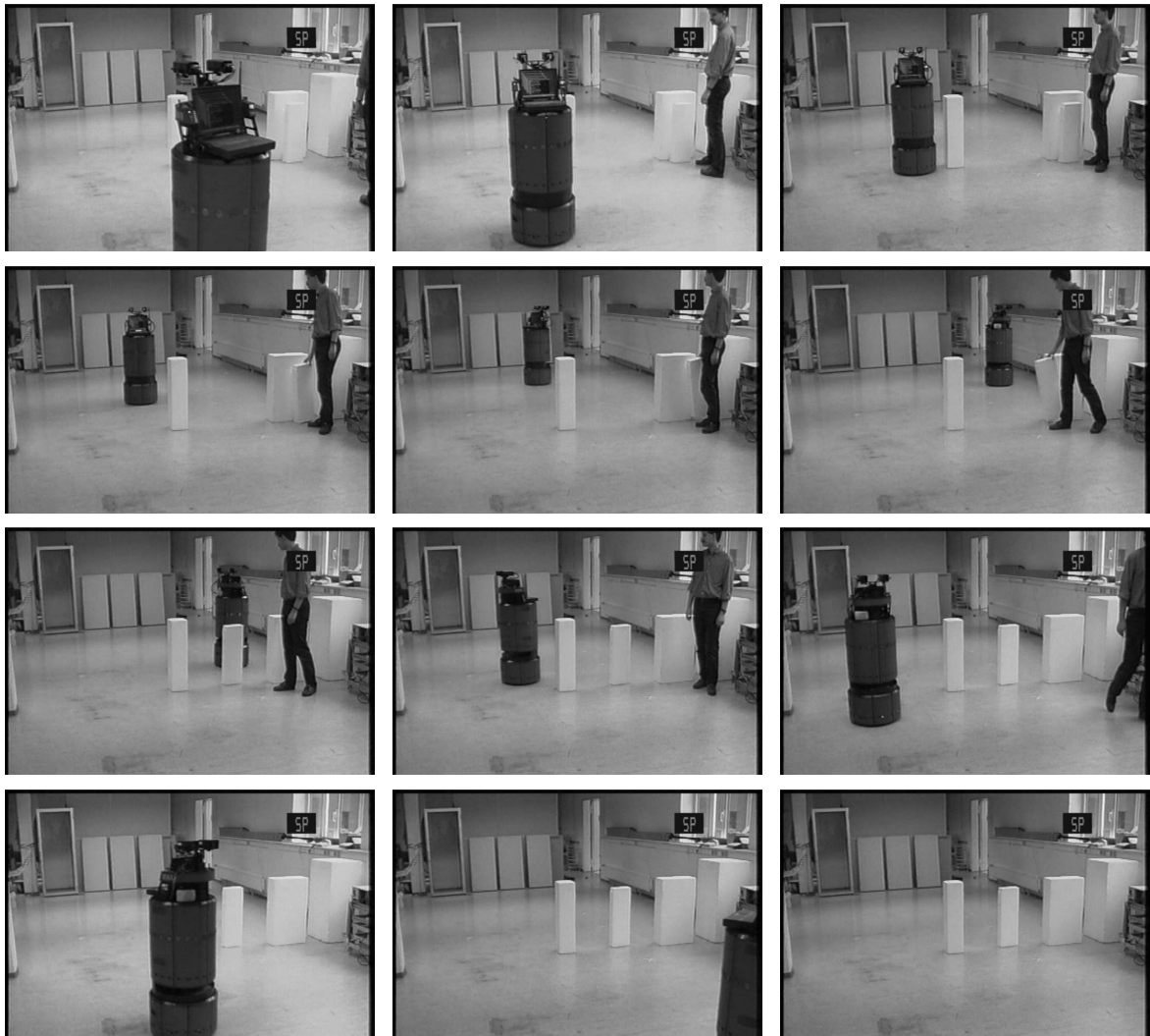
Figure 3.29: Provoking the robot to circumvent the obstacles by blocking the passage.
