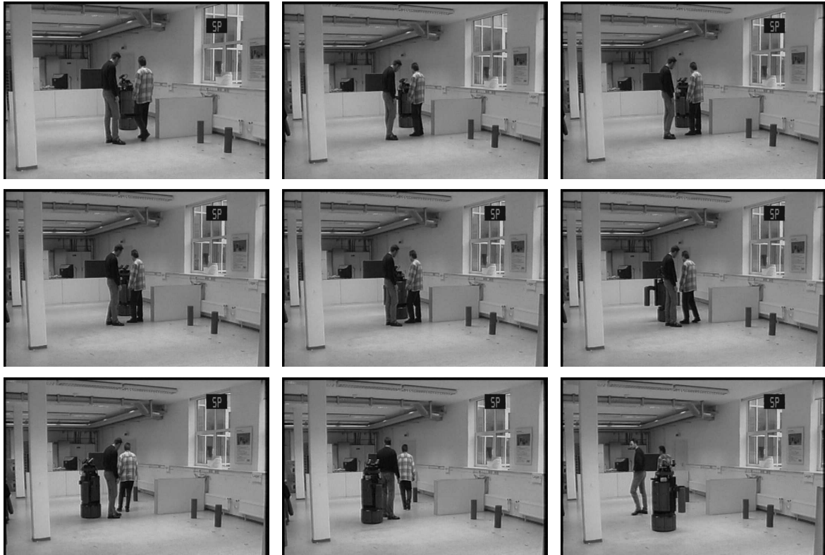
Figure 3.26: Causing the robot with a deployed manipulator to circumvent persons.
